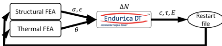
Fig.10. Endurica DT's co-simulation workflow updates the crack length c , exposure time \tau , and stiffness E so that stress, strain, and temperature fields can be updated during solution.
